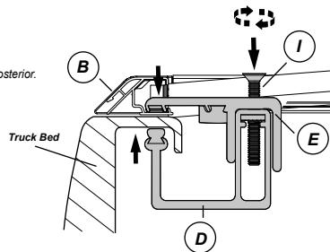
**NOTE:** When installing the clamps you may have to modify the bed-liner if present.
