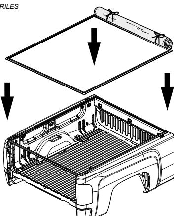
Position Rail Assembly onto the bed rails of the truck. Center assembly on rails. Loosely attach Clamp Assemblies.
