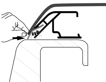
**Starting at the front, tuck plastic retainer on the cover into the Rail Channel. Work towards the back of the vehicle.**
