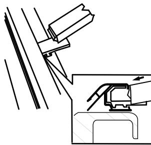
**Insert bows to rail assembly by resting the bow on the top of the slider tabs with each of its legs draped over the sides.**
