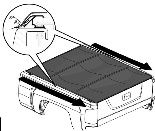
**Repeat step 5 for both side rails of the Tonneau Cover. Make sure all clamps are securely tightened, and all seals are set in the rail channel. Installation Complete.**
