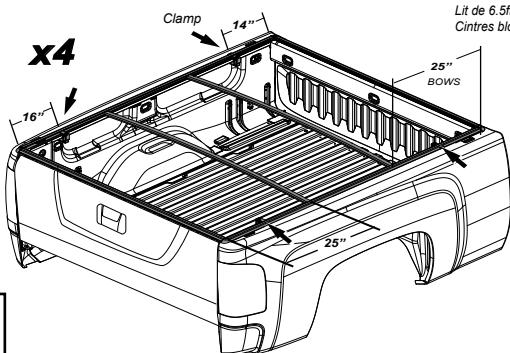
**NOTE:** When installing the clamps you may have to modify the bed-liner if present.
