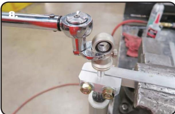
**8.** With the Tool still clamped on the shaft, thread the new upper mount onto the shock shaft. Use a Crows Foot on a Torque Wrench to tighten the new Upper Mount. The mount should be tightened to correct torque for the mount you are installing. See Torque Specifications below.
