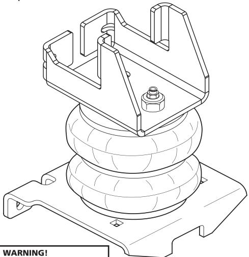
Do not inflate this assembly when it is unrestricted. The assembly must be restricted by the suspension or other adequate structure. Do not inflate beyond 100 P.S.I. Improper use or over inflation may cause property damage or severe personal injury.
