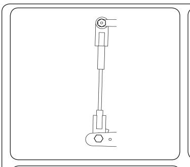
9. With the sensor and the axle bracket mounted, it is time to connect the 2 with the supplied linkage. The linkage is a universal length and will have to be cut to achieve the necessary length for your application. To do this it will be necessary to have the truck sitting at its factory ride height. With the truck at ride height center the sensor in its travel. The rod can slide into each rubber rod end up to 1".
