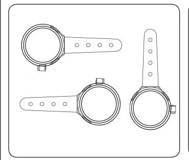
5. The Axle bracket can be mounted in any location on the axle tube to get the sensor linkage to line up. The Axle mount should be mounted on the axle so that the linkage will line up from the axle mount to the sensor. Keep this in mind when establishing the sensor location.
