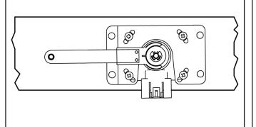
7. The sensor needs to be mounted on the frame rail with the wires pointing down. The arm will need to swing up opposite the direction of the wires as the suspension is being compressed. Attach the sensor bracket to the frame with (4) self drilling screws supplied with the kit.
