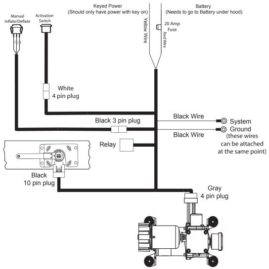
**Red Wire** - This wire needs to go straight to the **Battery** with the fuse holder installed within 18" of the Battery
