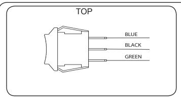
12. Hook the wires up to the manual control switch as shown in the diagram.
