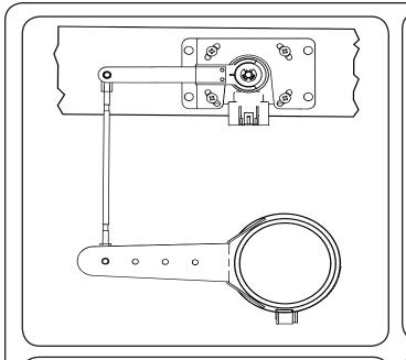
6. The next step will be to mount the sensor. The Smart Sensor needs to be centered in its travel at the trucks ride height to operate properly. This can be done by cutting the linkage rod to length. It can be fine tuned by loosening the 4 sensor mounting screws and twisting it in the mount and retightening the 4 screws. When the mounting and linkage is done it should look like the diagram seen here.
