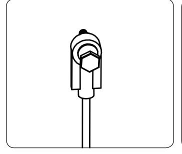
10. The linkage rod has barbs on the outside of it to keep it in the end link. After you push the ends in, they are difficult to pull back out. Push the linkage into the ends a little at a time until you get the desired length of the linkage assembly. If for some reason you must pull the rod out of the end, it is best done by twisting the end while pulling on it.
