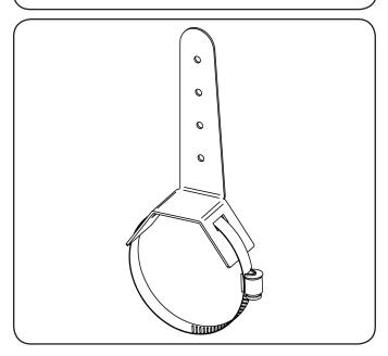
8. This diagram shows how the clamp sticks through the axle bracket. Loosen the clamp until it will open up and then slide it through the bracket. The whole assembly can then be put on the axle tube. Reinsert the end of the clamp back into the adjuster and tighten the clamp until the bracket is tight on the axle tube.
