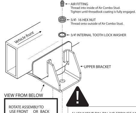
ALIGNMENT PIN ON AIR SPRINGS MUST BE INSTALLED TO FULLY SEAT INTO ONE OF THE ALIGNMENT HOLES IN THE UPPER BRACKET. FAILURE TO DO SO WILL CAUSE IT TO BE PUSHED INTO THE BEAD PLATE, CREATING AN AIR LEAK, AND RESULTING IN AN AIR SPRING FAILURE THAT IS NOT WARRANTABLE. THE ALIGNMENT PIN CANNOT HOLD 2,500 LBS! IT IS USED FOR ALIGNMENT ONLY!
