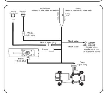
2. Unpack the wiring for the LevelTow system and lay it out. This will give you an idea to where you can mount the components without having to modify the wiring harness.
