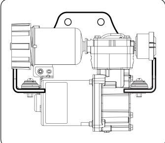
4. The compressor needs to be mounted on the frame rail with the dryer up. Attach the compressor bracket to the frame with (4) 3/8"-16 x 1" Thread Forming Bolts supplied in the kit. Drill a 5/16" Hole for the bolts.
