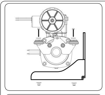
3. Bolt the compressor to the bracket. Position the compressor on the Bracket in the orientaion shown. Line up the holes in the (4) Mounting Bushings with the (4) holes in the Bracket. Install a #10 Flat Washer on each of the (4) #10-24 x 1 1/4" Pan Head Screws. Insert a Screw/Washer in each of the 4 holes. Install a #10 Flat Washer on the threads sticking through the bottom of the bracket followed by a #10-24 Nylok Nut. Tighten the hardware.
