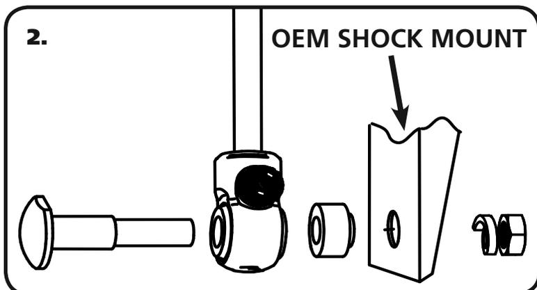
2. The Lower Shock is Bolted to the Lower OEM Mount using the supplied Cantilever Pin. Insert the Threaded Pin into the 5/8" Sleeve installed in the shock. Slide the supplied Spacer onto the threads of the Pin and insert the assembly into the OEM shock hole. Install the 1/2" Split Lock Washer onto the threads sticking through the the OEM mount, followed by the supplied 1/2"-20 Nut. Tighten the Hardware.
