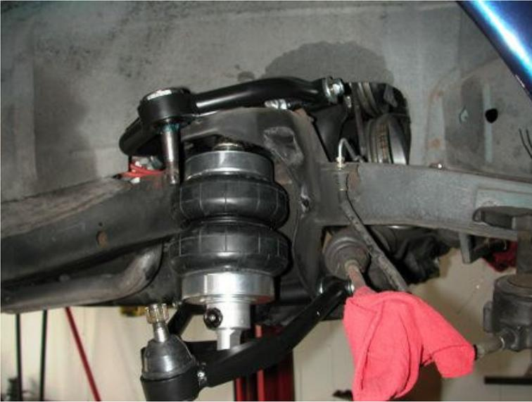
1. Fasten the upper arm to the frame using the factory hardware. Reinstall the current alignment shims, but **vehicle must be realigned.**
