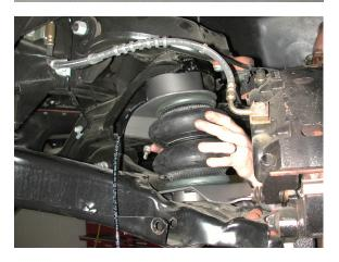
5. Insert airline into fitting and install the airspring and bracket assembly into the front suspension as shown. Note that the upper bracket "tongue" will be inside the crossmember as shown below. The lower bracket will be positioned by the oem sway bar hole in the lower control arm.
