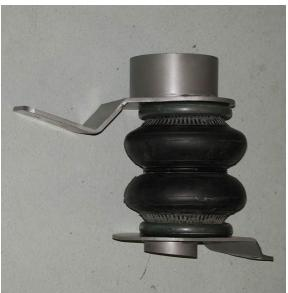
4. Assemble the upper and lower brackets onto the airspring as shown to the left. This is the driver side assembly as viewed from the front. Be sure to install the airline fitting into the airspring and position it so the airline has a clear exit to the side of the upper cup.
