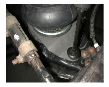
7. This photo shows how the lower bracket is positioned by the oem sway bar mount.
