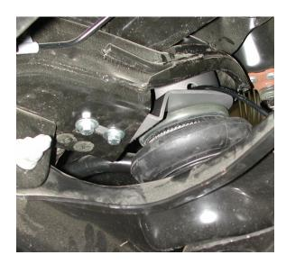
6. This photo shows how the "tongue" of the upper bracket is inserted into the trucks crossmember and bolted down.
