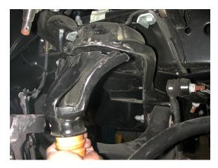
3. The Dodge has a large protrusion that extends from the upper coil spring pocket that supports the compression bump stop. This protrusion will be trimmed off. This can be accomplished with a cutoff wheel, torch, or a sawzall.
