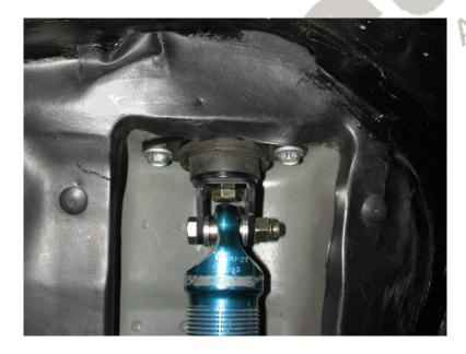
6. Bolt the eyelet to the lower control arm using the 1/2" x 3" bolt and Nylok nut. An aluminum .4375" thick spacer must be installed on each side of the bearing.
