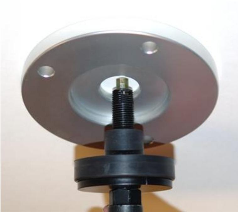
4. Bolt the aluminum upper plate to the car in place of the factory rubber mount using the 3/8" x 1 1/4" bolts, flat washer and Nylok nuts.
