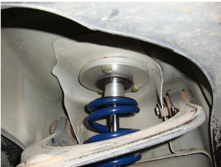
6. From the engine bay, place the other rubber bushing over the stud, then another steel plate. Secure the assembly with a 9/16" SAE Nylok Jam nut. **Note:** Some cars may have a plastic cover in the engine bay that may need to be clearance for the adjustment knob.
