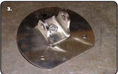
**3.** Using the 7/16-14" x 1" Hex Bolt and 7/16"-14 Nylok Nut bolt the Upper Shock Mount to the Upper Mounting Plate. The 7/16" Bolt needs to be installed with the Hex Head of the bolt in the Shock Mount. The shock mount needs to clocked on the mounting plate. The edge of the Shock Mount needs to be positioned parallel with the edge of the Mounting Plate. Tighten the 7/16" Bolt and nut keeping the shock mount clocked correctly.
