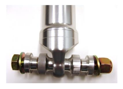
5. Fasten the Shockwave to the lower control arm with a 5/8" x 5" bolt, Nylok nut and flat washers. The aluminum spacer and T-bushings must be installed as shown.
