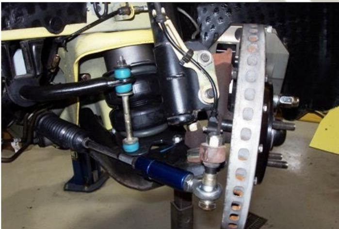
10. Reattach the sway bar end link to the lower control arm.
