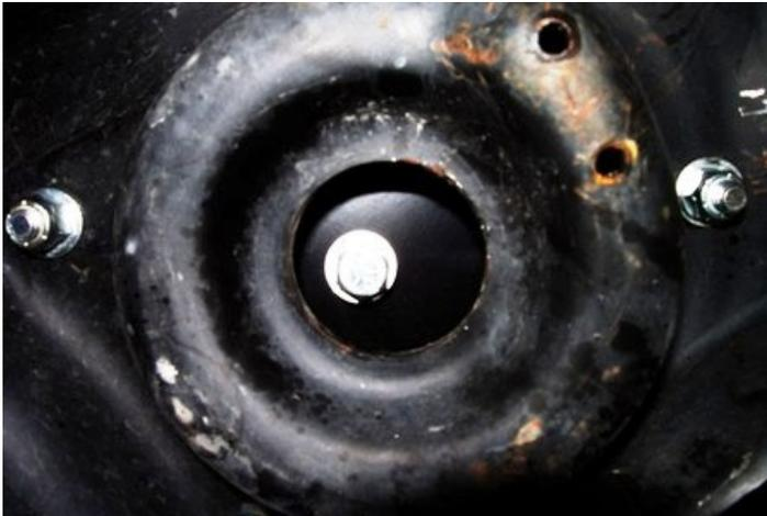
9. Fasten the air spring to the lower plate using a 3/8" x 1" bolt, lock washer and flat washer.
