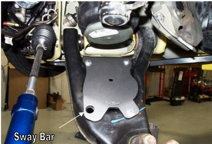
3. Place the lower air spring plate on top of the lower control arm. They are labeled D for driver and P for passenger.
