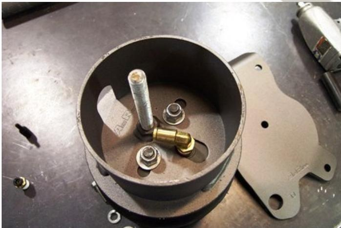
5. Apply thread sealant to the a 90 degree air fitting and screw it into the top of the air spring.
