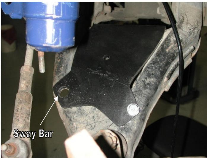
3. Place the lower air spring plate on top of the lower control arm. They are labeled D for driver and P for passenger.
