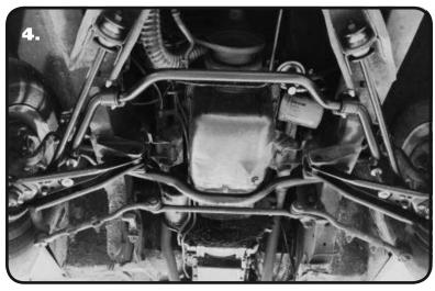
**4.** Slide the SwayBar into position on the Car. The SwayBar Arms will be above the Control Arms. Slide the Front Hole of the SwayBar Bushing onto the 3/8"-16 Stud. Hold it in place with a 3/8" SAE Flatwasher and 3/8"-16 Nylok Nut. Install the Correct Lockwasher and Flatwasher on the Correct Hex Bolt. Do **NOT** Completely tighten the Hardware. It will be left partially loose until the End Links are installed.
