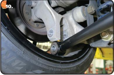
**10.** Insert the outer end of the lower control arm into the knuckle of the rear suspension. Align the bolt hole of the outer knuckle with the inner sleeve of the lower control arm.
