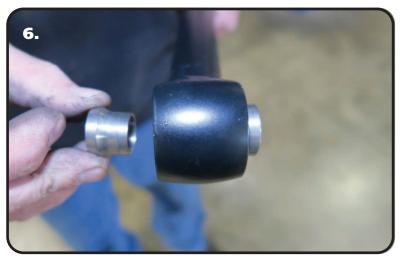
**6.** Install R-joint Spacers into the inner R-joint. Install the Spacers by inserting the SMALL side of the SPACER into the Center Pivot Ball. Push them in until they bottom out and stop.
