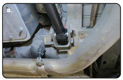
**8.** Insert the R-Joint end of the lower control arm into the inner mount. Make sure it is installed with the outer end angling to the front of the car.
