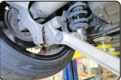
**4.** Remove the bolt from the outer end of the lower control arm and remove the control arm.
