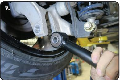
**7.** If you are installing the lower control arms with the wheels/tires still on the car, insert the outer end of the lower control arm into the wheel, below the knuckle.
