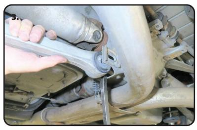
**3.** Remove the adjuster cam from the inner mount of the lower control arm. Remove the inner end of the control arm from the mount. We used a pry bar between the frame mount and lower control arm to help pry it out.
