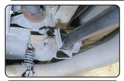
**9.** Reinstall the cam adjuster. Use the marks from **Step 2** to put the adjuster back in the same position as it was removed from. Torque to 186 ftlbs.
