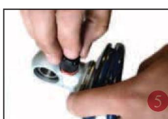
Install upper spring mount retainer clip (90002057) into the groove on the upper eyelet as seen in figure 5. Then reinstall adjuster to complete assembly.
