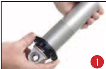
First using the supplied lower adjuster nut(90002222) thread the nut onto the shock from the bottom side as seen in figure 1
