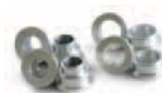
The included set of bearing spacers (900002044) are used to adapt the coil-overs to just about any application. The supplied spacers allow the coil-overs to accept 5/8" or 1/2" bolts.
