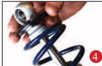
Slide the Derlin washer over the spring, Next slide the upper spring mount (90002222) over eyelet as seen in figure 4.
