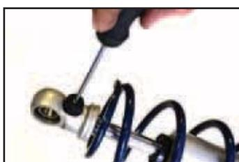
Before the upper spring mount can be installed screw the adjuster knob on the upper eye mount to the firmest setting (clockwise) as seen in figure 3.
