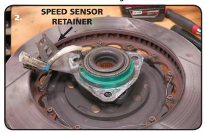
2. Even if you purchased new Hub Bearings, the existing Speed Sensor Plug Retainer will need to be reused. The Plug Retainer is positioned between the spindle and hub bearing. To get to it, the Hub Bearings will need to be disassembled from the OEM spindle. Remove the (3) Bolts attaching the hub to the spindle.
