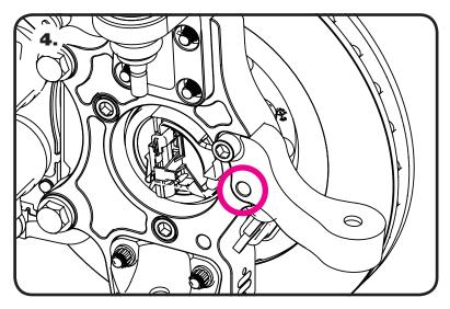
**4. REAR ONLY-** The Rear will require the Emergency Brake Cable Mount to be attached to the Ridetech Modular Spindle. Remove the Mount from the OEM Spindle. Remove the **BOTTOM** Bolt from the Steering Arm of the new spindle. The Hole is circled in **Image 4**.
