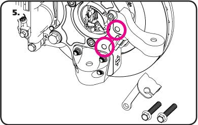
**5.** The OEM Cable Mount will align with the (2) holes circled in **Image 5**. Use **Images 5 & 6** to aid in the installation of the mount.
