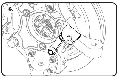
**6.** Attach the Cable Mount to the Spindle using the OEM Hardware. Apply RED Loctite to the threads of the bolts before installing. Install the Bolts while holding the Mount in position. Torque the Bolts to 40 ftlbs.
