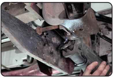
**6.** The rear of the leaf springs will need to be disconnected to install the new hanger setup and to move the springs under the axle. Support the rear of the leaf spring and remove the leaf spring shackle bolt. If your truck has a hitch on it, you will find it easier to cut the bolt to remove it from the shackle/hanger.
