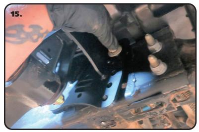
**15.** Determine the set of holes that you are going to be using to attach the hanger. The hanger is bolted to the frame in the OEM location with the open side of the shackle to the front of the truck. The REAR UPPER hole reuses the OEM bolt that was removed earlier. Install the OEM bolt in the rear upper hole. This will help hold the hanger while inserting the remaining bolts.
