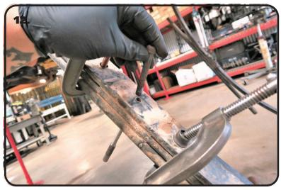
**12.** Remove the locating pin from the leaf spring pack. Reinstall the locating pin from the TOP side. Reinstall the nut on the BOTTOM side and tighten. With the nut tight, remove the clamps. Repeat on the second spring.
