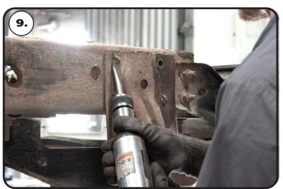
**9.** The rear leaf spring hanger will need to be removed from the frame. It is held on by (1) bolt and (3) rivets. Remove the bolt from the top rear hanger hole. We remove the rivets by cutting a " + " in the rivet head and chiseling if off. After chiseling the head off, drive the rivet out of the hanger/frame with a punch.
