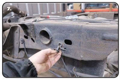
**7.** Unbolt the emergency brake cable bracket from the driver side frame rail. It is located between the axle and the front leaf spring hanger. Retain the hardware for reassembly.
