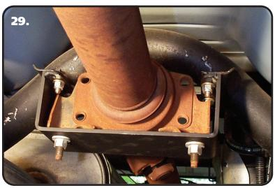
**29.** The new carrier bearing bracket is then bolted onto the remaining tabs. Attach the bracket using 3/8"-16 x 1" bolts, flat washers, & 3/8"-16 nylok nuts. The carrier bearing mount is rotated 180 degrees and attached to the supplied bracket with the OEM hardware as shown in the picture in **Image 29**.
