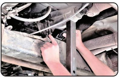
**26.** The kit includes a transmission spacer that will need to be used to help with driveline angles. Install it by loosening the hardware that attaches the transmission mount to the transmission crossmember. Jack up the rear of the transmission just enough to slide the spacer in and tighten the hardware.
