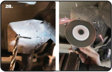
**28. Image 28** illustrates drilling and cutting the OEM carrier bearing mount. Drill the (4) marked holes using a 3/8" drill bit. Cut along the line that was marked along the inner edge of the new mount. This will remove the center of the OEM mount.
