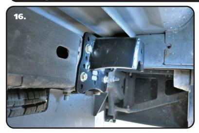
**16.** Install a 7/16" flat washer on each of (3) 7/16"-14 x 1 1/4" bolts. Align the correct holes of the hanger with the OEM holes in the frame. Install a bolt/washer in each one. Install a 7/16" flat washer and 7/16"-14 nylok nut on the threads of the bolts that are sticking through the frame. Torque the hardware to 70 ftlbs.
