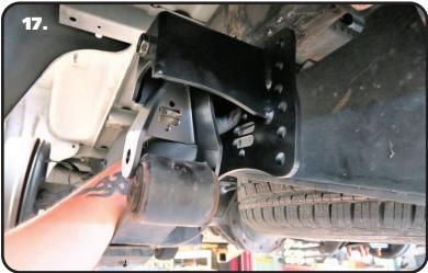
**17.** Raise the rear of the leaf spring up until it lines up with the rear shackle. You may have to jack up the rear differential. Install the OEM hardware that was removed earlier. Repeat on the second spring. Do not tighten the hardware at this time.
