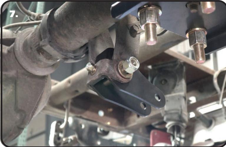
**7.** Install a 9/16" flat washer on a 9/16"-18 x 3 1/4" Bolt, insert the bolt/washer through the lower mount, OEM mount, and spacer. Install a 9/16" Washer and 9/16"-18 Nylok Nut on the threads sticking through the mounts/spacer. Tighten the 5/16" hardware to 25 ftlbs. Tighten the 9/16" hardware to 100 ftlbs. Repeat for the other shock bracket.
