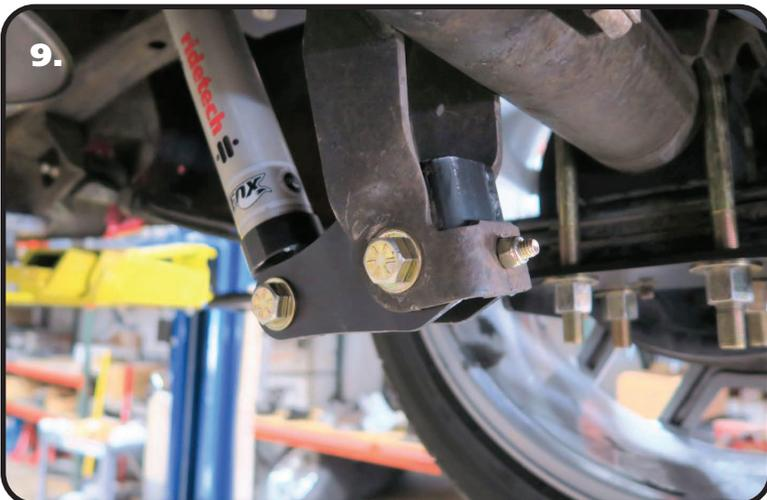
**9.** Install a 1/2" flat Washer on a 1/2"-13 x 2 3/4" Bolt. Line the center of the inner sleeve of the shock with the mounting holes in the lower shock bracket. Insert the bolt/washer through the lined up holes. Install a 1/2" Flat Washer and 1/2"-13 Nylok Nut on the threads sticking through. Torque to 50 ftlbs.
