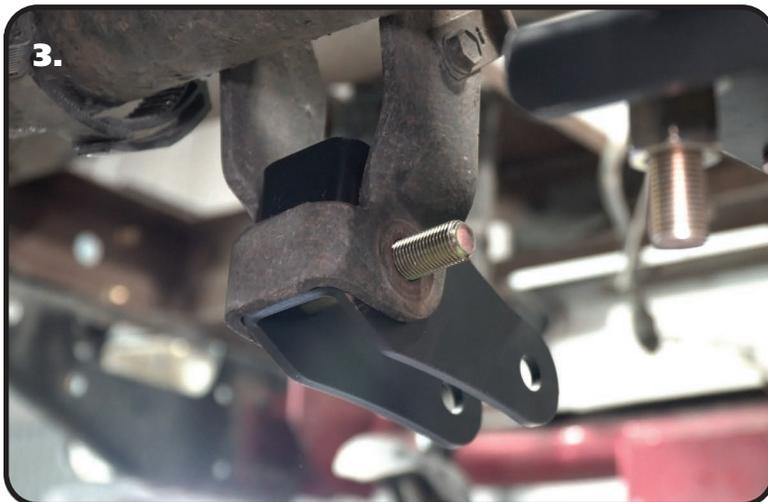
3. This kit includes new lower shock mounts to correct the angle of the shocks. They attach to the OEM shock mounts. Slip the lower mount into the OEM shock mount lining up the 2 side holes with the OEM shock hole. You will need to drill the rear hole into the OEM mount. Use the bracket as a template to mark the location of the hole that will need to be drilled.
