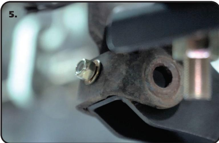
5. Reinstall the new shock mount, aligning the holes. Install a 5/16" Flat Washer on a 5/16"-18 x 1" Bolt and insert in through the small hole with the bolt head on the INSIDE of the new shock mount. Install a 5/16" flat washer followed by a 5/16"-18 Nylok Nut on the threads of the bolt sticking through the bracket. Do not tighten at this time.
