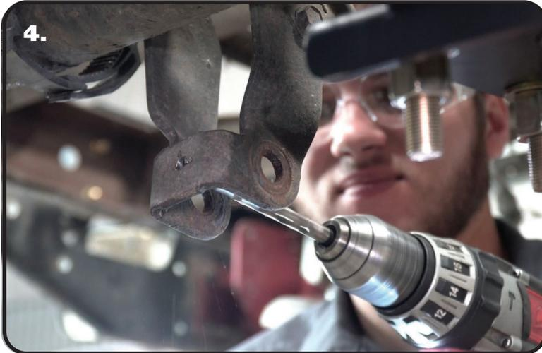
4. You will need to remove the new mount to be able to drill the hole in the OEM mount. Use a 5/16" drill bit to drill the hole.
