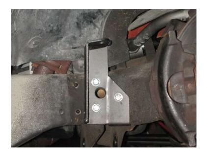
1. The large hole in the bracket will align with large hole in the frame. Using the bracket as a template, drill the remaining holes in the frame. Use 3/8" x 1 1/4" bolts, Nylok nuts and washers to secure the bracket. The inside of the frame can be accessed from the coil spring pocket to install the nuts.
