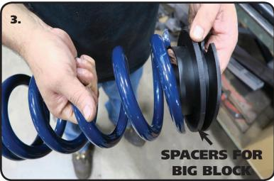
**3.** The CoilSpring Seat is positioned on the top of the Coil Spring with the ring inserted into the CoilSpring. **Small Block requires NO Spacers**. **Big Block trucks require 2 Spacers on the Spring Seat**.
