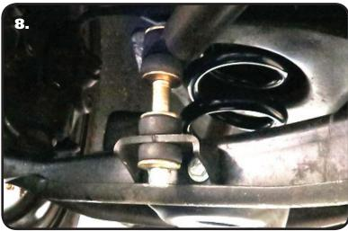
**8.** Install a 3/8" Flat Washer on (2) 3/8"-16 x 1 1/4" Hex Bolts and insert them into the holes. Install a 3/8" Flat Washer and 3/8"-16 Nylok Nut on each Bolt. Repeat on the other side and tighten hardware.
