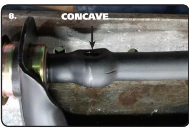
**8.** Reattach Control Arms to Truck. Use the OEM Hardware to attach the Lower making sure the Locating Pin for the lower cross shaft is in the hole. The Pin in the Cross Shaft Saddle will locate into the Holes. The Upper Control Arm Cross Shaft has a Concave area around the bolt hole. This Concave needs to go against the Convex Spacer on the Cross Shaft Bolts. The shims go behind the convex spacer. Reattach the Upper Control arms using the OEM Hardware and installing the Alignment Shims.
