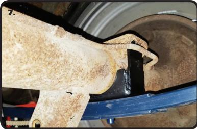
**7.** Lower the Differential down into the Flip Brackets. The Tabs that stick up will rest against the OEM leaf spring mount. This keeps the axle from slipping in the Bracket.
