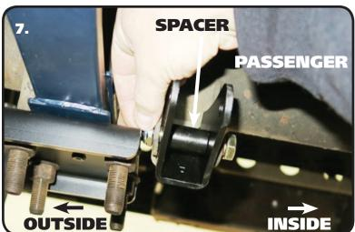
7. The kit includes a spacer that goes inside the New Bracket. Install the 1/2" ID spacer into the Bracket lining it up with the OEM shock holes and holes in the Bracket. Insert a 1/2"-20 x 2 1/2" Bolt through the lined up holes with the THREADS TOWARD THE WHEEL. Install a 1/2"-20 THIN Nylok Nut. Do this for both Shock Mounts. Tighten the 1/2" & 7/16" Hardware on both mounts.
