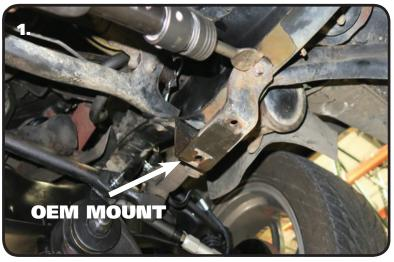
1. Some trucks are equipped with a sway bar. If your truck has one, the OEM mount will need to be removed to install the Street-Grip Sway Bar. This is done by removing the rivets. The rivets can be removed by chiseling the heads off and driving them out or by drilling the rivets out. The new Frame Mount bolts directly in place of the old mount. If your truck doesn't have a sway bar, the mounting holes will still be in the frame.
