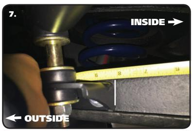
7. This kit requires a Bracket to be installed on the control arm for the sway bar linkage. The Bracket needs to be positioned with the inside edge 8" from the CONTROL ARM BUSHING and the ears pointing DOWN. Hold the end of the tape measure against the outer edge of the Control Arm Bushing and make a mark on the Control Arm at 8". Hold the Bracket on the Control Arm with the ears pointing DOWN and against the lip of the control arm. Use the bracket to mark and drill the mounting holes to 3/8".
