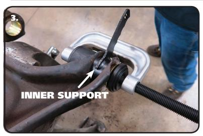
3. LOWER CONTROL ARM: The Lower Control Arm's Outer Shells can be installed before the Cross Shaft is installed, it will slide through the Shells. We used a C-clamp style tool to install our bushings. Most auto parts stores have these as a loan-a-tool. When pressing the Outer Shell into the arm, be sure to support the inside of the arm to keep it from crushing. Press the shell in until it bottoms against the control arm.
