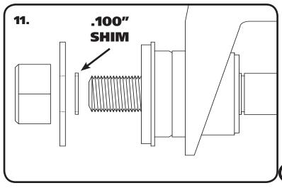
11. The nut and washer will need to be removed from the rear bushing. Slide the shim or shims onto the rear threads of the cross shaft. Install the nust and washer and tight until the washer is against the bushing. Check to see how if the gap has been elimated. If there is less than 1/16", tighten the upper cross shaft nuts to elimate it. After the gap has been elimated, refer to Step 8 of the previous page for control arm reattachment to the truck.
