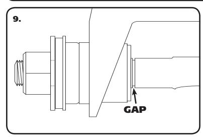
**9.** We have ran across variances in the width of the upper control arms. Typically .100" or .200" wider. We provide (4) .100" shims in the kit to take up the gap. When installing the shims, they need to be installed in the rear bushing. Start by loosening the rear nut and tightening the front until the cross shaft bottoms against the bushing/inner sleeve. There may be a gap between the rear inner sleeve and the cross shaft. If this gap is larger than 1/16", shimming will be required.
