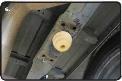
**6.** Install the Bump Stop using a 3/8" Flat Washer & 3/8"-16 Nylok Nut. Hold the Bump Stop with your hand while tightening the nut.
