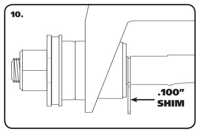
**10.** With the cross shaft tightened against the front bushing/inner sleeve, use the supplied shims to determine how much shim is needed to fill the gap. Typically, 1 or 2 shims will be needed. Hold the shim up to the gap to see how much is needed.
