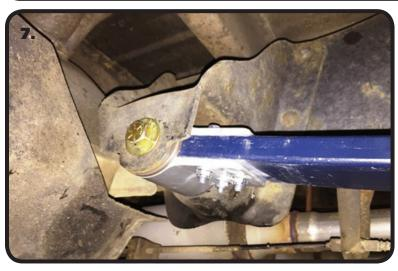
**6.** Swing the front of the Leaf Spring up into the front Hanger aligning the Differential with the Flip Bracket. It may be necessary to raise the Differential up to get the Leaf Spring into the front hanger. Align the holes in the Hanger with the Bushing Sleeve. Install a 9/16" Flat Washer on a 9/16"-12 x 4 1/2" Bolt supplied in this kit. Insert the Bolt/Washer through the Hanger & Leaf Spring. Install a 2nd 9/16" Flat Washer & 9/16"-12 Nylok Nut on the Threads sticking through.
