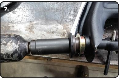
7. Push the Inner Sleeve into the Delrin Bushing. Push the Delrin Bushing/Inner Sleeve assembly into the Outer Shells. They will go in partially. Install the OEM washer and nut on each end of the cross shaft. Tighten the Hardware on each end until the Delrin Bushings are bottomed out against the lip of the Outer Shell installed in the control arm.
