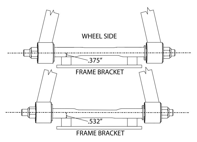
The cross shaft that is used in the upper control arms is offset. The offset combined with the caster slug option allows you to achieve the alignment setting you desire with minimal shims. To change the direction the Icon faces simply spin the cross shaft in the control arm.
