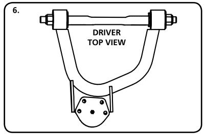
**6.** Diagram "6" shows the Driver Upper Control Arm. This is looking at the control arm from the top.
