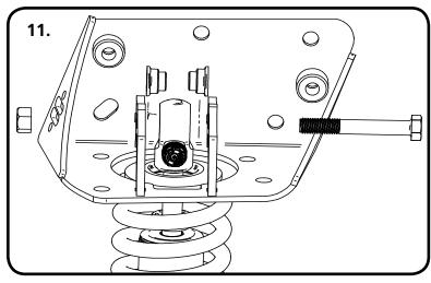
**11.** Install a spacer on each side of the upper Shockwave/Coilover. Slide the assembly into the upper mount from the bottom side. If your shock has an adjuster knob position it to the wheel side of the mount. Line up the hole in the spacers with the hole in the strap and insert 1/2" x 3 1/4" bolt and install 1/2" Nylok nut.
