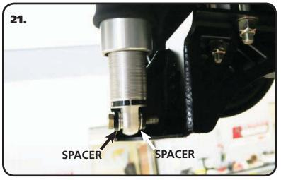
21. Insert a Spacer into each side of the lower Shockwave/CoilOver bearing. Slide the shock, with the spacers installed, into the mount on the Lower Axle Mount. You may need to jack the rearend up to line up the holes in the bushings with the 1/2" hole in the shock mounts and hold it in place while you install the 1/2" x 2 1/2" Bolt and 1/2" Nylok Nut with a 1/2" SAE Flat Washer on each side of the mount. Tighten the upper and lower shock bolts to 75 ftlbs.
