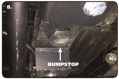
**8.** Install the bumpstops into the "C" Notches using a 3/8" nut and flat washer. Tighten the hardware enough to hold the bumpstop in place.
