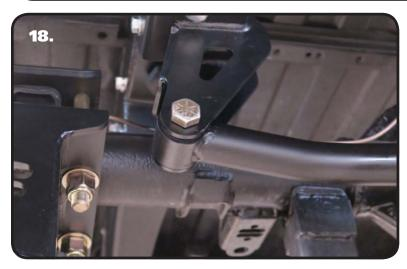
**18.** Install the Panhard bar into the frame bracket. The Panhard Bar is a bent bar, it is bent to clear the center section of the rear differential. The bar needs to be mounted with the BEND to the REAR and the Rubber Bushing in the Frame Mount, this will help it clear the differential cover. The Panhard bar is attached using (1) 5/8" x 3" bolt, (1) 5/8" Nylok Jam Nut & (2) 5/8" Flat Washers. Tighten the hardware enough to eliminate any gaps.
