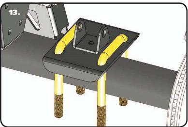
**13.** The Kit includes 2 Upper Bar Mounts that are the same. Each one sits on a leaf spring pad with the center pin indexed into the center hole of the leaf spring pad. Sit an Upper Bar Mount on top of the axle with the locating pin into the center hole of the leaf spring pad. Install a 5/8" Square U-bolts through each pair of side holes in the Upper Bar Mount with the threads pointing down. The U-bolts will run parallel to the frame.
