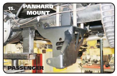
**15.** Repeat the above step on the Passenger Lower Mount. Torque the hardware to 60 ftlbs in a crisscross fashion.
