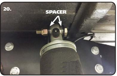
**20.** Insert a Spacer into each side of the upper Shockwave/CoilOver bearing. Slide the assembly into the upper shock mount. If your shock has an adjuster knob, position it so that the knob points toward the outside of the truck. Line up the hole in the spacers with the hole in the upper shock mount and insert 1/2" x 2 1/2" bolt and 1/2" Nylok nut with a 1/2" SAE Flat Washer on each side of the mount.
