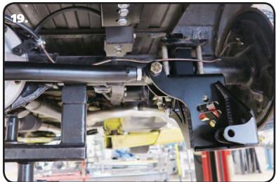
19. Install the R-Joint Spacers into the Center Pivot Ball of the R-Joint in the Panhard Bar. Install the other end of the Panhard bar into the mount on the Passenger Lower Axle Mount. The Panhard bar is attached using (1) 5/8" x 3" bolt, (1) 5/8" Nylok Jam Nut & (2) 5/8" Flat Washers. Tighten the hardware enough to eliminate any gaps.
