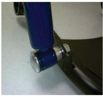
3. Slide the lower shock stud through shock, then install the aluminum spacer. The step on the spacer will face the lower arm. Secure the stud to the lower arm w/ the ½" flat washer and nut.
