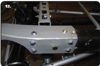
12. Once both "C" Notches are in place bolt in the upper shock bridge. The new upper shock bridge uses the (3) holes in the top of the "C" Notch. The bridge is offset to the rear of the truck, it goes from "C" Notch to "C"notch under neath the top lip of the frame sandwiching the frame between it and the "C" Notch. It is bolted in place using (6) 7/16" x 1 ¼ bolts, Nylok nuts and flat washers.
