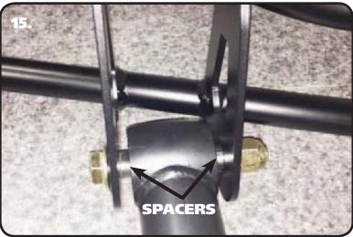
**15.** The StongArms are a direct replacement of the factory trailing arms an will bolt to the new tubular cross member using two 5/8" x 4 1/2" Bolts, 4 Flat Washers, & 2 Nylok nuts. Insert the R Joint Spacers into each side of the R Joint. These bushings are Delrin and do NOT need lubricating.
