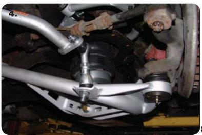
**4.** Attach the Posilinks in the **CENTER** hole of the MuscleBar and the StrongArm using a 7/16" SAE Flatwasher on each side of the arm on the MuscleBar and each side of the bracket on the StrongArm. Install 12mm Nylok nut on each posilink and tighten down.
