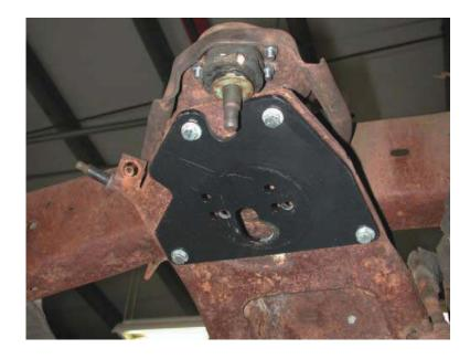
1. Hold the upper plate to the cross member as shown in the picture to the left and clamp to frame. Using the plate as a template drill four 3/8" holes in the cross member.
