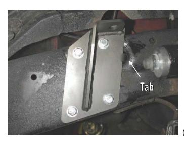
1. Place the new upper shock mount against the frame, the tab in the front of the bracket will slide into the factory shock stud hole. Position the bracket so that the bottom of the bracket is parallel to the bottom of the frame. Using the bracket as a template, mark an drill four 3/8" holes in the frame rail. Secure the bracket to the frame using four 3/8" x 1 ¼" bolts, Nylok nuts and flat washers.
