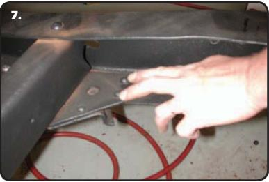
**7.** On the driver side of the rear frame cross member; these two rivets must be removed before installing the "C" notch. Also, remove the factory panhard mount.
