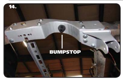
**14.** Install the bumpstops into the "C" Notch using a 3/8" nut and flatwasher.
