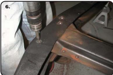
**6.** The factory upper shock cross member must also be removed to allow for the new upper shock cross member and "C" Notch.
