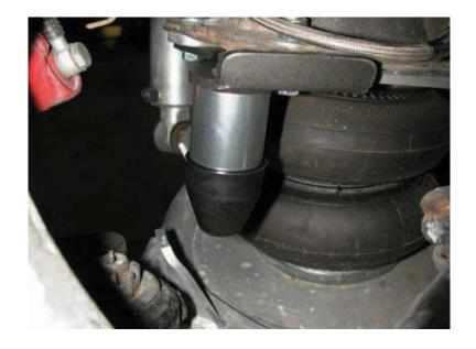
**Note**: It is acceptable to let the suspension bottom on the air spring. However, if your tire hits the inner fender well before the air spring bottoms out, this bump stop must be installed.
