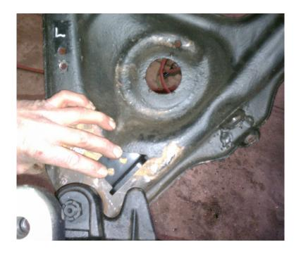
6. Use the Image as a reference for placing the steering stop. It should be parallel with the rear edge of the control arm. You want the steering stop of the spindle to hit the steering stop before the steering box hits the internal stop. Use the stop as a template to drill (2) 3/8" holes in the control arm. Attach the stop using (2) 3/8"-16 x 1 1/4" bolts, (4) flat washer, & (2) 3/8"-16 nylok nuts.
