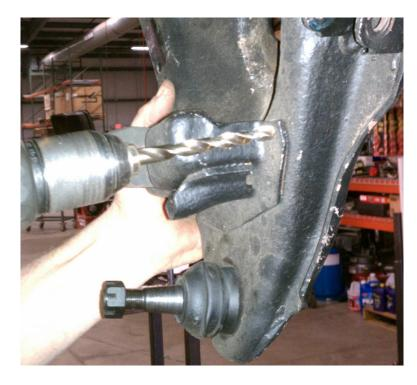
5. Use a drill to drill the spot welds out of the OEM bumpstop/steering stop. Just drill through the mount. Do NOT drill through the control arm. We recommend cleaning the area up after removing it and paint it to keep the area from rusting.
