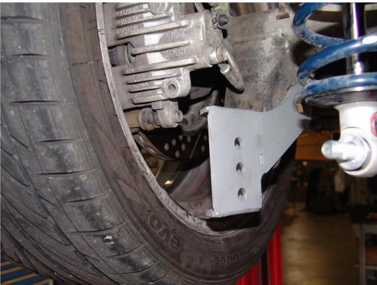
6. Remove the lower trailing arm mounting bolt. (Do one side at a time to keep the axle from rotating).
