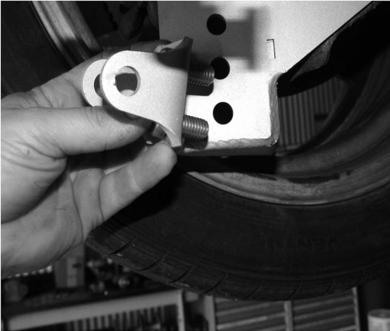
8. Install the Lower Bolt on Shock Bracket in the top 2 holes using (2)  $\frac{1}{2}$ " x  $1\frac{1}{2}$ " Hex Bolts, and (2)  $\frac{1}{2}$ " Nylok Nuts.
