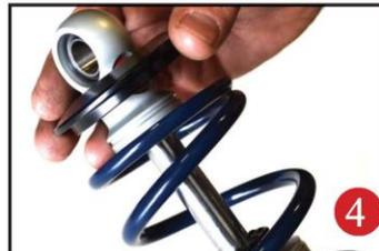
Slide the Delrin washer over the spring, Next slide the upper spring mount (90002222) over eyelet as seen in figure 4.
