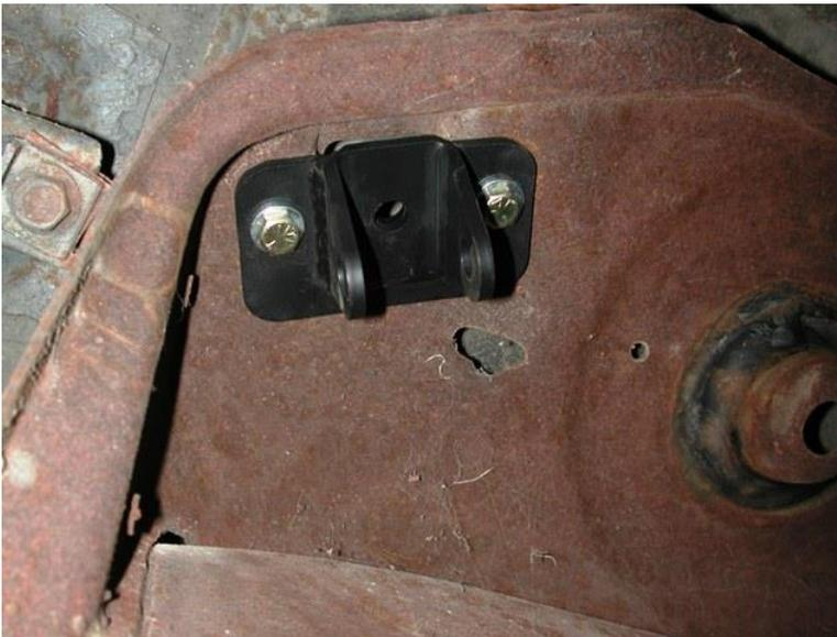
5. Fasten the new upper shock bracket into the factory shock location using the 5/16" x 1" bolts, flat washers and Nylok nuts supplied.
