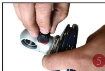
Install upper spring mount retainer clip (90002057) into the groove on the upper eyelet as seen in figure 5. Then reinstall adjuster to complete assembly.
