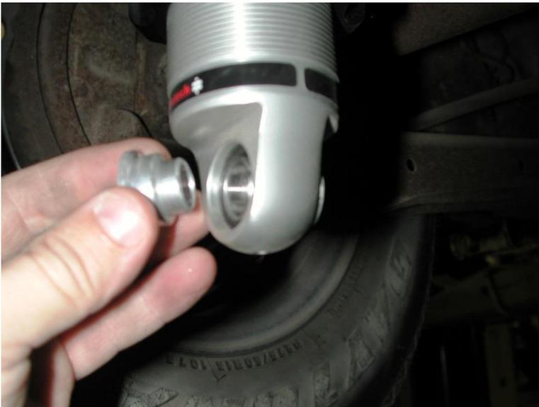
9. Install the aluminum spacers into the upper and lower eyes of the shock.
