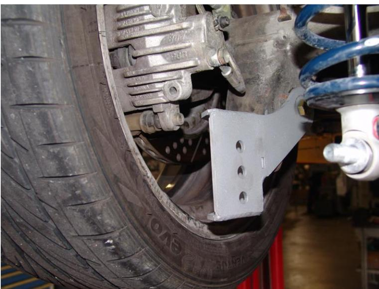
6. Remove the lower trailing arm mounting bolt. (Do one side at a time to keep the axle from rotating).
