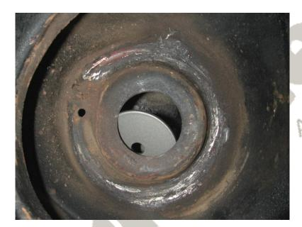
4. Place the upper washer on top of the coil spring pocket.
