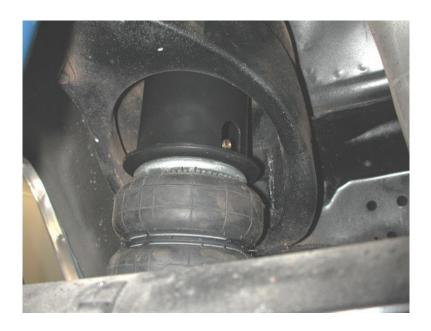
5. Raise the assembly into the coil spring pocket with the all thread sticking through the upper washer. Secure the assembly with a 7/16" Nylok nut and flat washer.
