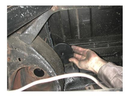
1. If you have a large hole in the coil spring retainer you will need to place the large upper washer on top of the frame to attach the upper cup bracket.
