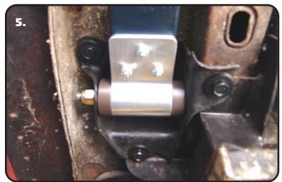
**5.** Swing the Leaf Spring up and attached the front mount to the car using the supplied 3/8"-16 x 1 1/2" Conical Body Bolts and U-Nuts. Tighten Hardware
