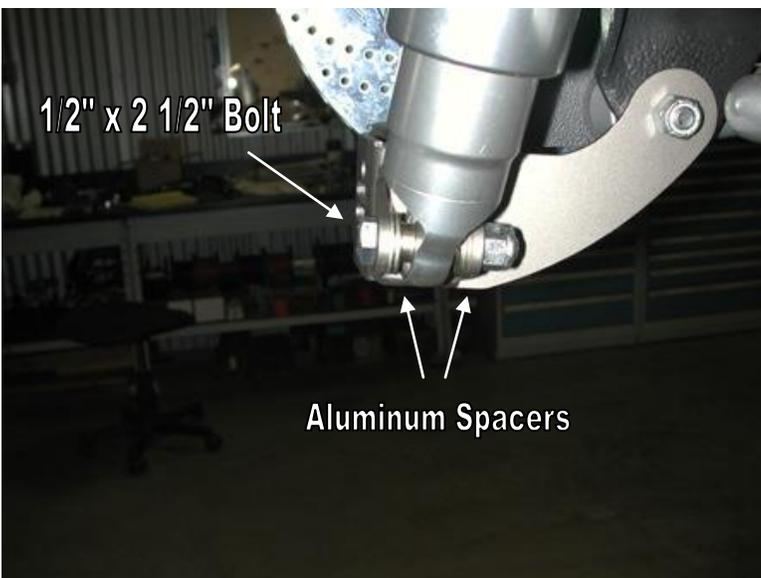
11. Fasten the CoilOver to the lower bracket using a 1/2" x 2 1/2" bolt and Nylok nut. 1/2" I.D. aluminum spacers must be installed on each side of the bearing.
