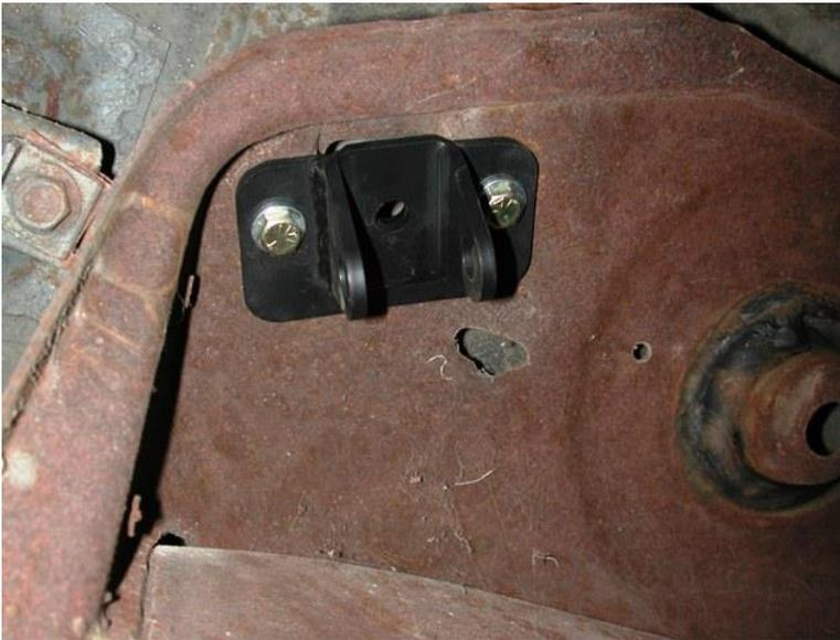
8. Fasten the new upper shock bracket into the factory shock location using the 5/16" x 1" bolts, flat washers and Nylok nuts supplied.
