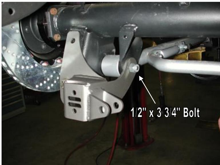
4. Remove the lower trailing arm mounting bolt. (Do one side at a time to keep the axle from rotating).
