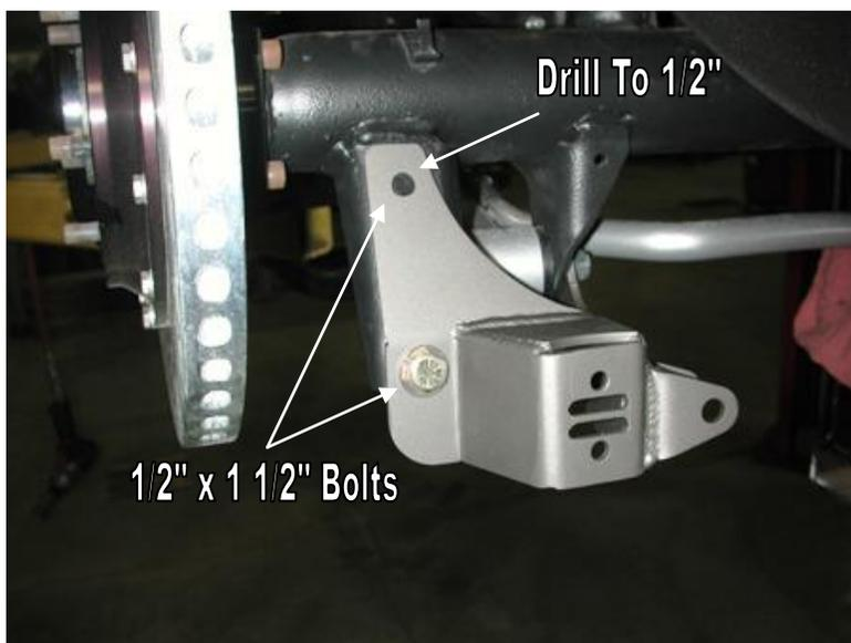
6. The lower bolt hole in the back of the bracket will align with the factory shock stud hole. Use a 1/2" x 1 1/2" bolt, Nylok nut and flat washers.
