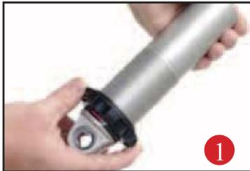
First using the supplied lower adjuster nut (90002222) thread the nut onto the shock from the bottom side as seen in figure 1
