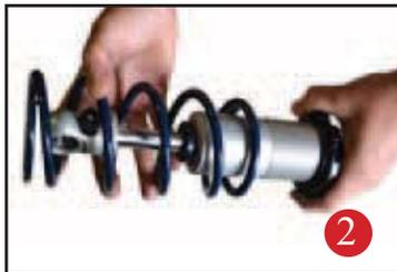
Next install delrin washers then coil spring over the top of the shock as seen in figure 2
