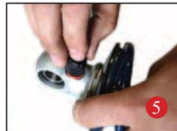
Install upper spring mount retainer clip (90002057) into the groove on the upper eyelet as seen in figure 5. Then reinstall adjuster to complete assembly.
