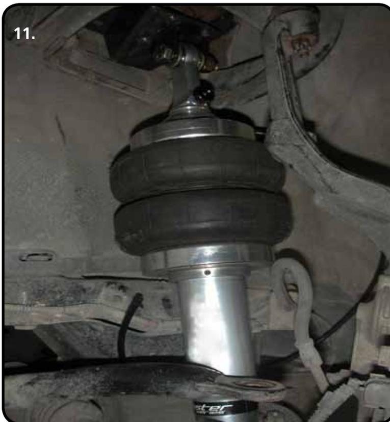
**11.** Route the Air line to the Valves. Be sure to stay away from heat sources and sharp edges.
