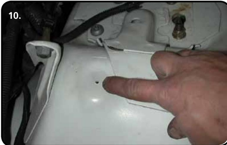
**10.** A bump stop will be installed between the inner fender and upper control arm to ensure that the tire does not hit the inner fender when fully compressed. There is a small hole on the inner fender that must be drilled out to 3/8". Fasten the bump stop to the inner fender using a 3/8" Nylok nut and flat washer.
