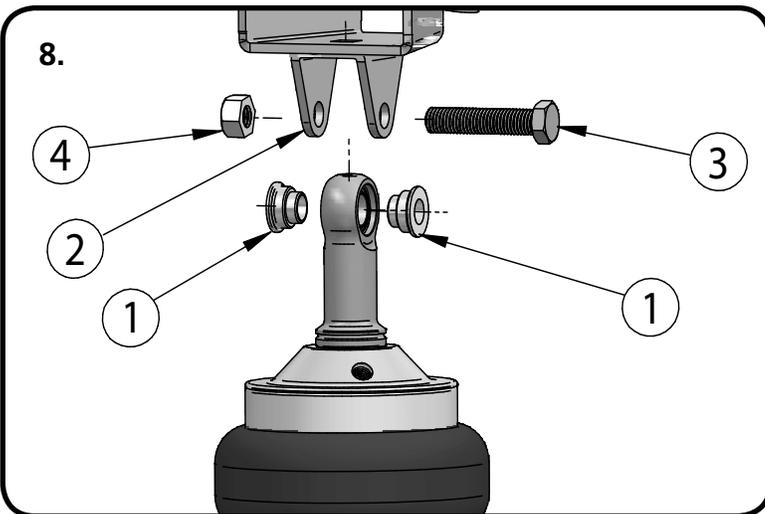
8. Thread the fitting into the ShockWave using Teflon tape on the threads. Assemble the spacers(1) into the bearing in the upper eyelet. With the spacers installed insert the ShockWave assembly into the upper shock mount(2). Align the holes in the bracket with the hole in the Shock spacers and insert the 1/2" Bolt(3) and secure with the 1/2" Nylok Nut(4).
