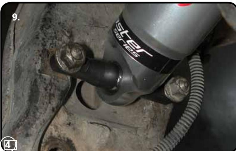
9. Attach the lower ShockWave mount to the OEM Lower Control Arm using (2) 3/8"-16 x 3" Bolts, (4) 3/8" Flatwashers, and (2) 3/8"-16 Nylok Nuts. Tighten Hardware. It may be necessary to raise the lower control arm up to align the ShockWave Trunnion with the OEM Mount.
