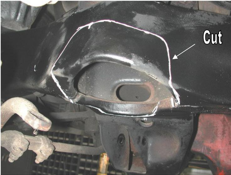
1. The frame pocket must be trimmed to ensure that the air spring does not rub against the frame. The coil spring retaining “fingers” must also be trimmed.
