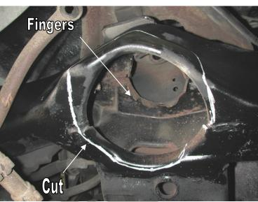
1. The frame pocket must be trimmed to ensure that the air spring does not rub against the frame. The coil spring retaining "fingers" must also be trimmed.
