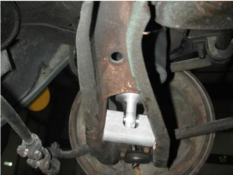
11. Bolt the billet mount to the lower control arm use a 3/8" x 4" bolt, Nylok nut and flat washers.
