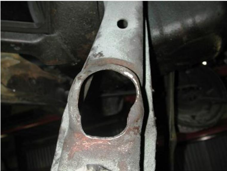
6. Grind edges smooth and paint exposed metal on lower control arm.
