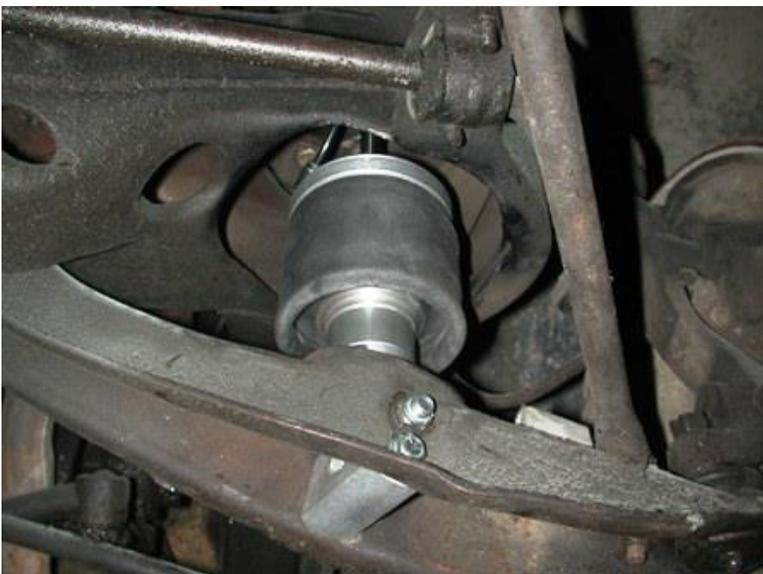
13. Double check Shockwave clearance through full suspension travel. **Allowing the Shockwave to rub will result in failure** and is not a warrantable situation.
