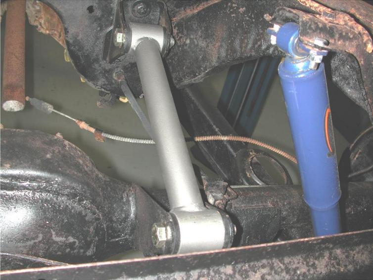
1. Insert the LONG R-joint Spacers into the R-joint. The Small Diameter goes into the R-joint. Bolt the upper StrongArm to the frame using the 5/8" x 3 1/2" bolts and Nylok nuts supplied.
