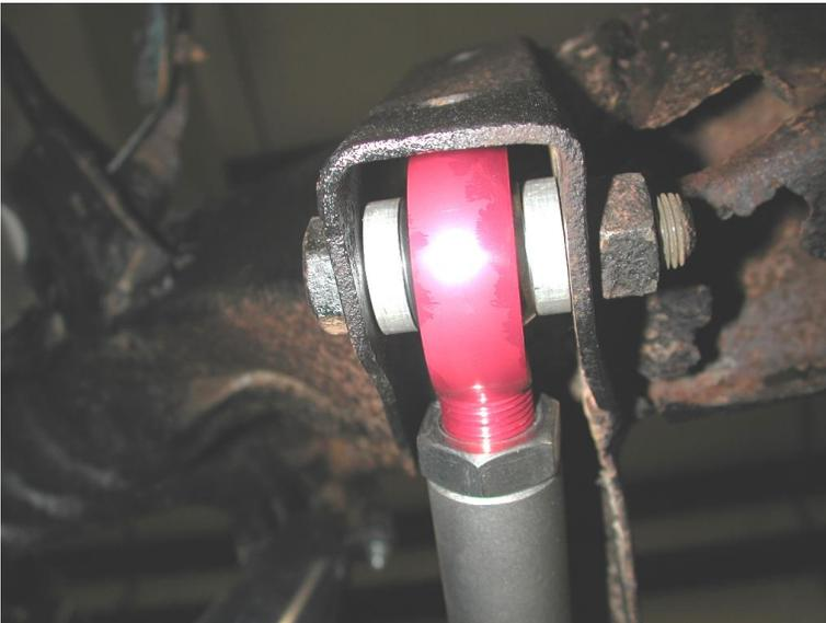
3. Install the 3/4" jam nut onto the end of the Heim end, then screw Heim end into the end of the panhard bar.
