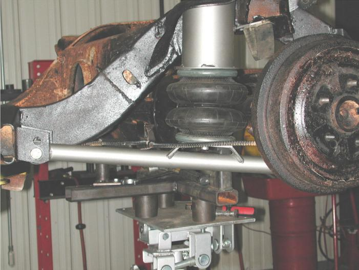
2. Fasten the lower StrongArms to the frame and axle using the 5/8" x 3 1/2" bolt and Nylok nuts supplied.
