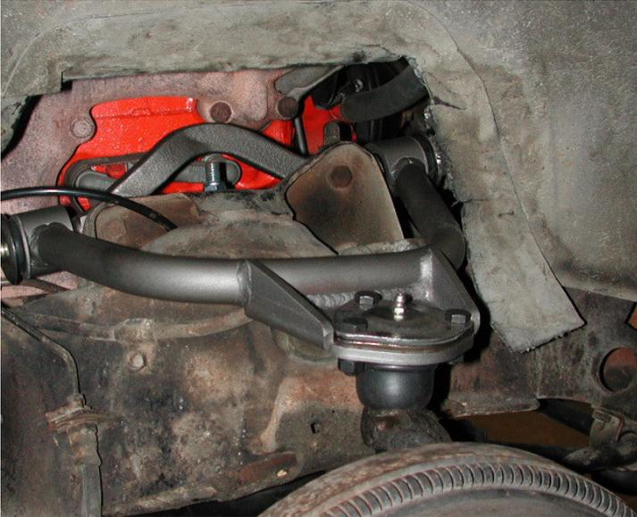
1. Drop the ball joint down through the ball joint plate, secure w/ the hardware supplied.
