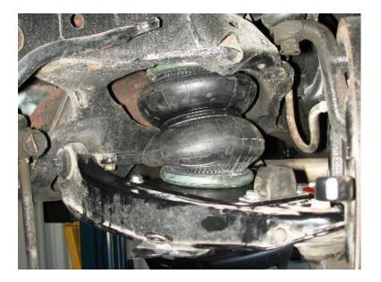
3. Bolt the lower air spring plate to the lower arm. The two outer holes will align with the factory bump stop holes. The inner two holes must be drilled.
