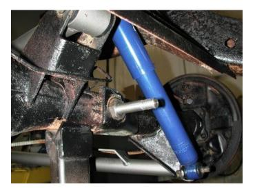
2. Attach the bottom of the shock to factory shock stud using the ½" Nylok nut & flat washer supplied supplied.
