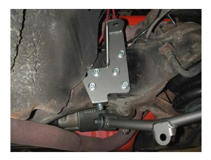
1. Position the upper shock mount on the frame so the hole in the bracket aligns with the hole in the side of the frame and the tab is against the bottom of the frame. You may have to trim some of the inner fender well for clearance. On manual shift cars you may have trim the bottom of the Z-bar clutch bracket on the driver's side.
