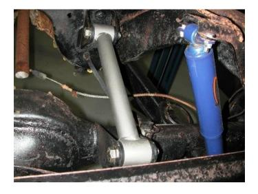
1. Attach shock T-Bar to frame using 5/16" x 1" bolts, Nylok nuts and flat washers.
