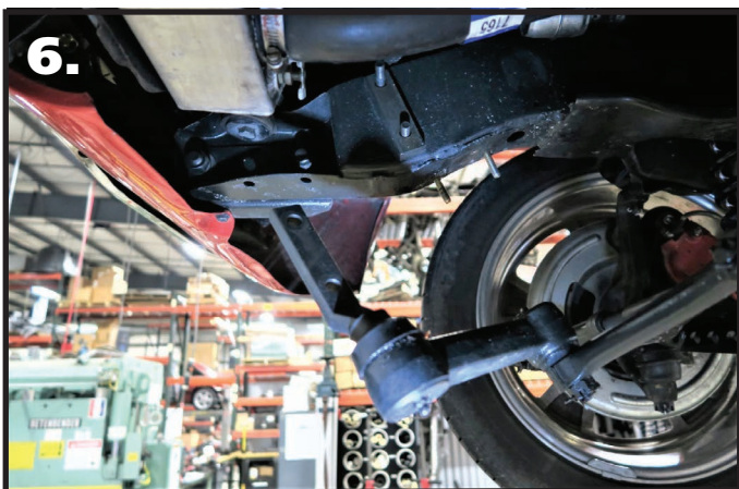
6. Disconnect the idler arms from the frame.
