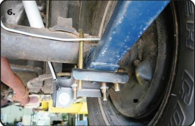
**5.** Bolt the **NARROW BUSHING END** of the Composite Leaf Spring into the OEM front leaf spring mount using a 1/2"-13 x 4" Hex Bolt and 1/2"-13 Nylok Nut.
