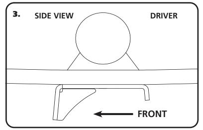
**Composite Leaf Spring Note:** When tightening the mounts, pay attention to the pads on the springs to make sure there is visible compression of the pads. .030"- .060" of compression is needed for the springs to be securely mounted. All of the clamping force needs to be on the spring itself.
