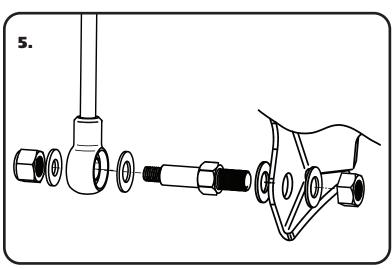
**6.** The Lower Shock is Bolted to the Lower Shock Mount using the supplied Shock Stud. Insert the Shock Stud into Lower Mount with a 5/8" Flat Washer on EACH side of the mount. Install a 5/8" Lock Nut on the threads and tighten. Next, slide a Washer on the Shock Stud. Jack the Rear Differential up until the Shocks can be slid onto the Shock Studs. Install a 7/16" Flat Washer and 7/16" Hex Nut onto the Threads and tighten.
