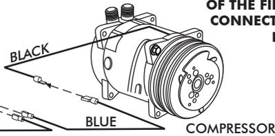
**NOTE: CONNECT WHITE WIRES DIRECTLY TO (-) BATTERY TERMINAL**
