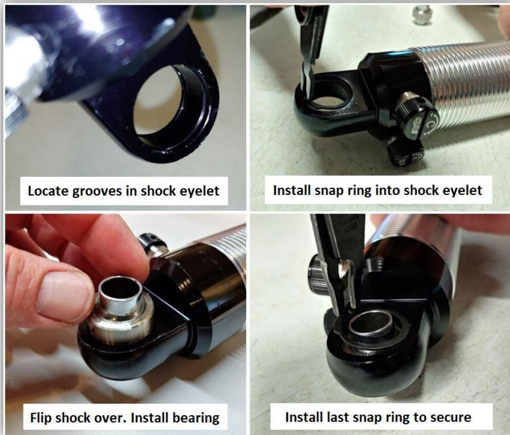
3. Install the coil-over shocks. Torque the shock mounting bolt to 70 lb. ft.
