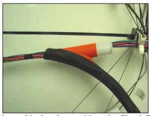
The "spreader" of the tool is then inserted into the ClassicBraid. With the tool inserted, pull the tool down the length of the ClassicBraid. This will insert the harness into the braid as it is pulled.
