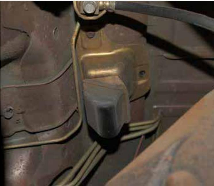
Locate pinion snubber bracket mounted to vehicle floor just above the front of the rear axle at the center of the vehicle.
