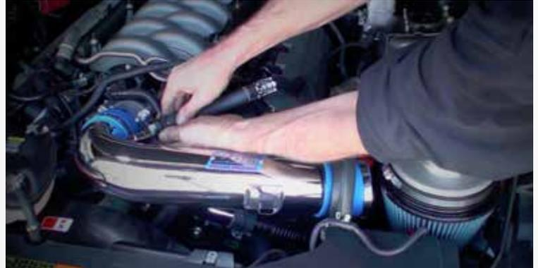
Disconnect the smaller plastic breather tube from the air inlet tube. You can leave the sound tube connected.
