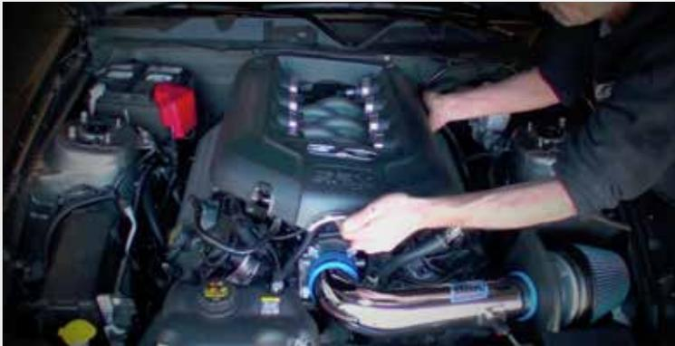
Remove the engine cover by pulling up on it to release its mounting pins from the grommets on the intake manifold.
