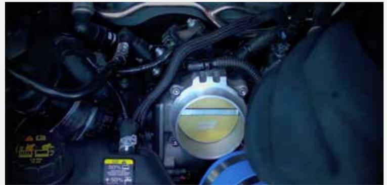
Re-install the air inlet tube and reconnect the breather tube. A little WD-40 or light grease on the inside of the tube may help in this process. Tighten the clamps.
