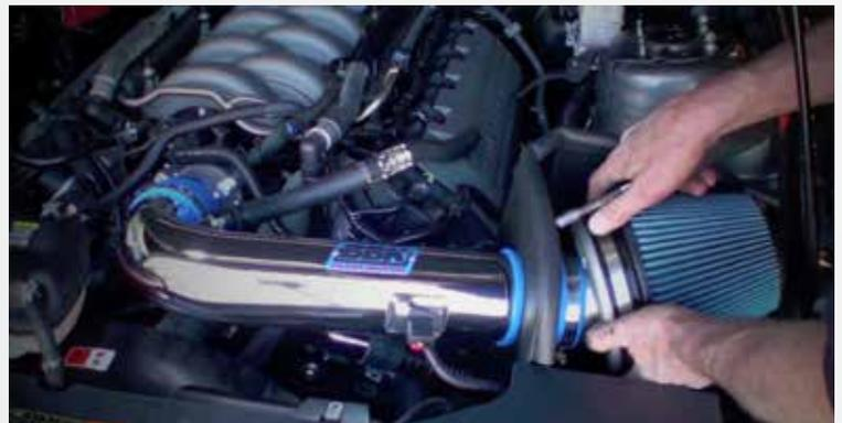
Remove the air inlet tube and set it aside.
