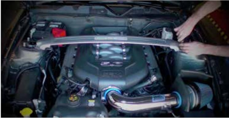
Remove the strut tower brace if applicable.
