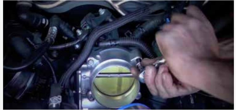
Connect the motor plug to the BBK Throttle Body and install onto the intake manifold. Use supplied bolts to secure the throttle body.
