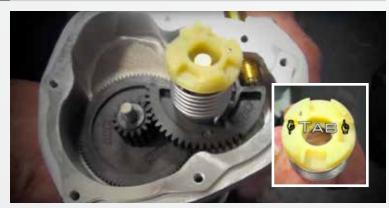
Place the plastic capped spring over the end of the throttle shaft of the BBK throttle body and line the pigtail hook on the spring up with the catch slot in the gear.
