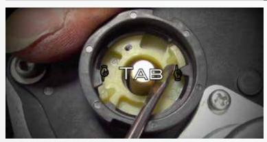
Using needle nosed pliers or screw driver rotate the plastic spring cap COUNTER-CLOCKWISE (approximately 180°) until the 2 tabs line up with their matching landings in the motor housing, then gently pull up on the cap until it pops up into a latched position.
