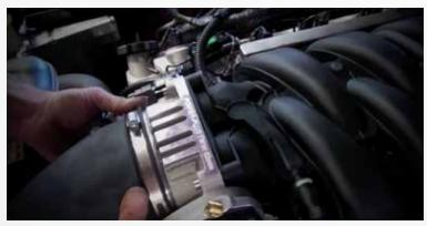
Re-install the intake hose and re-attach the PCV tube.
