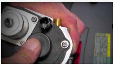
Align the tabs on the removable cap with the slots on the motor housing and snap it into place.
