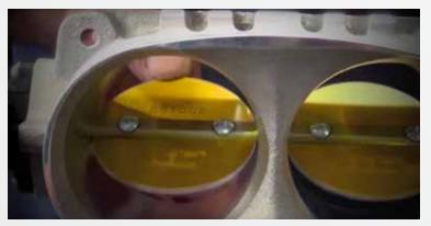
Check the throttle body for smooth action by opening and closing the flaps a few times with your fingers. You should feel a slight drag from the electric motor, but it should never bind or stick.
