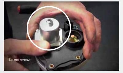
Install the motor housing minus the removable cap onto the BBK throttle body over the plastic spring cap and tighten screws.
