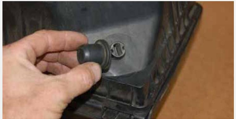
On the bottom rear of the stock air box, remove the rubber grommet for re-use with the BBK filter shield.
