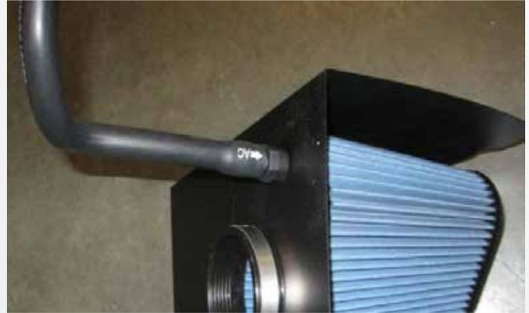
The 6.1L Engines require the use of the straight fitting for the breather hose.
