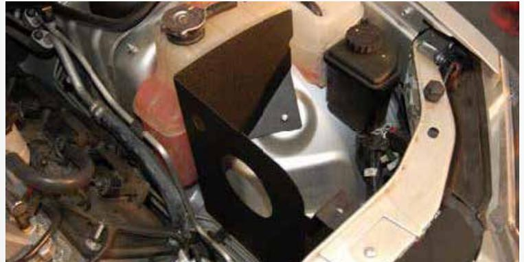
Place the filter shield into place in the engine compartment and line up the grommet with its hole. Mount the front tab of the filter shield using the stock bolt.
