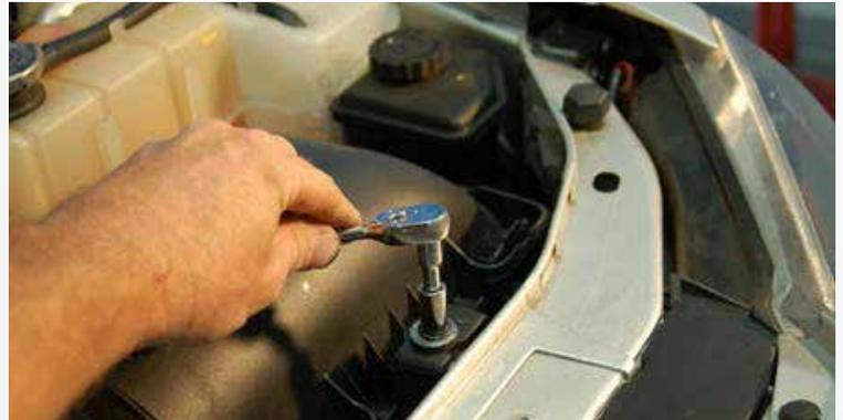
Remove the bolt that mounts the front of the air box to the vehicle. Lift out the air box and remove with the inlet hose.
