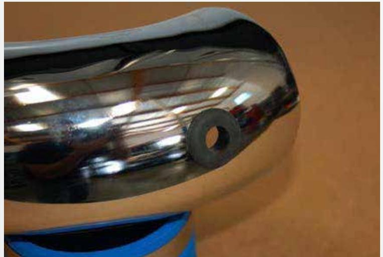
From the hardware kit, install the supplied rubber grommet into the hole in the BBK Inlet Tube. Install the Air Temperature Sensor into the grommet.
