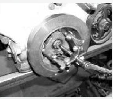
The stock balancer has three perches cast into it to facilitate use of a 3 prong puller tool. Hook the 3 prongs under the perches and use the bolt head as a pressure point for the 3 prong puller tool. Tighten the drive bolt on the puller tool until the balancer comes off of the crank snout completely.
