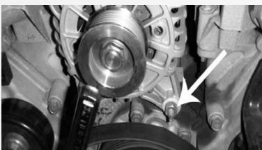
Before installing the BBK Water Pump Pulley the stud that supports the bottom right of the alternator needs to be removed and replaced with the supplied bolt. Now install the BBK Water Pump Pulley using the original bolts.
